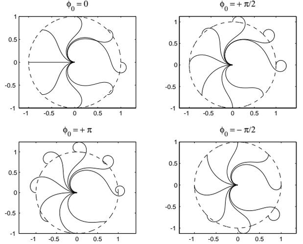
**Figure 2:** Paths starting on the unit circle with gains  $\gamma = 1$ ,  $h = 2$ ,  $\beta = 2.9$  and unsaturated linear velocity. From the top left in clockwise direction the starting orientation  $\phi_0$  is:  $0$ ,  $+\pi/2$ ,  $\pi$ ,  $-\pi/2$ .
