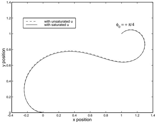
**Figure 5:** Paths with saturated (solid line,  $\bar{u} = 1/2$ ) and unsaturated (dashed line)  $u$  for the same initial configuration  $(1, 1, \pi/4)$  and same gains  $\gamma = 1$ ,  $\beta = 2.9$ ,  $h = 2$ .
