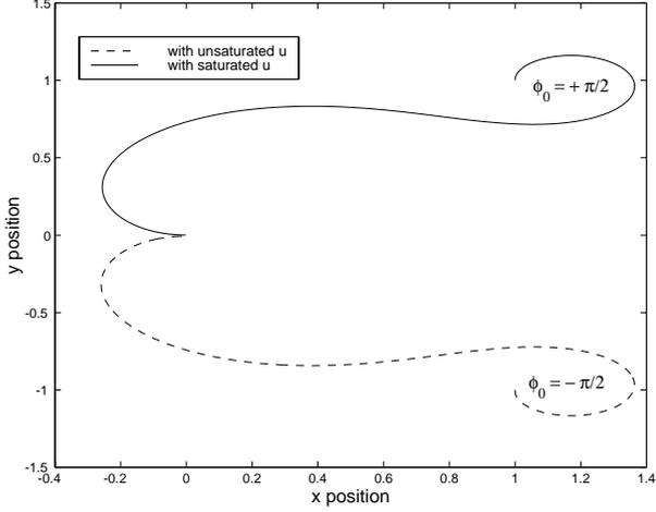
**Figure 3:** Paths with saturated (solid line,  $\bar{u} = 1/4$ ) and unsaturated (dashed line)  $u$  for symmetrical initial configurations and same gains  $\gamma = 1$ ,  $\beta = 2.91$ ,  $h = 2$ . The variables  $\alpha$ ,  $\theta$ ,  $\phi$ ,  $u$ ,  $c$  and  $e$  relative to this simulation are reported in figure (4).
