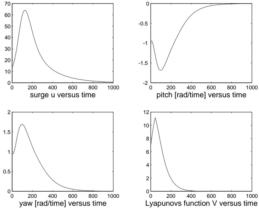
Fig. 5. Control inputs and Lyapunov function (6) relative to the path reported in figure (4). Notice that  $V$  is *not* always decreasing.
