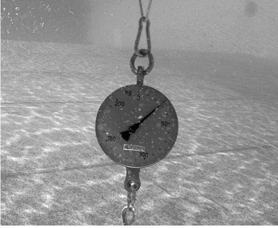
Fig. 10. Zoomed view of the picture reported in Fig. 9 showing the maximum (static) measured upward thrust.
