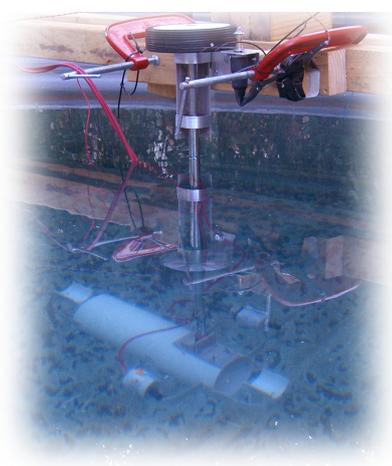
figure 5: Serafina mock hulls with the acoustic transducers
